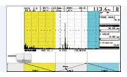
"Color Leg" indicator displays the legs of the angle beam inspection in different colors
